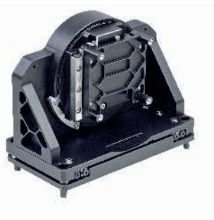
This three-axis system integrates two linear axes and a rotational axis and is used for aligning and fast, surface area scanning of photo-sensitive sensors. The use of PLine® ultrasonic motors makes shorter process times and a small installation space possible.
