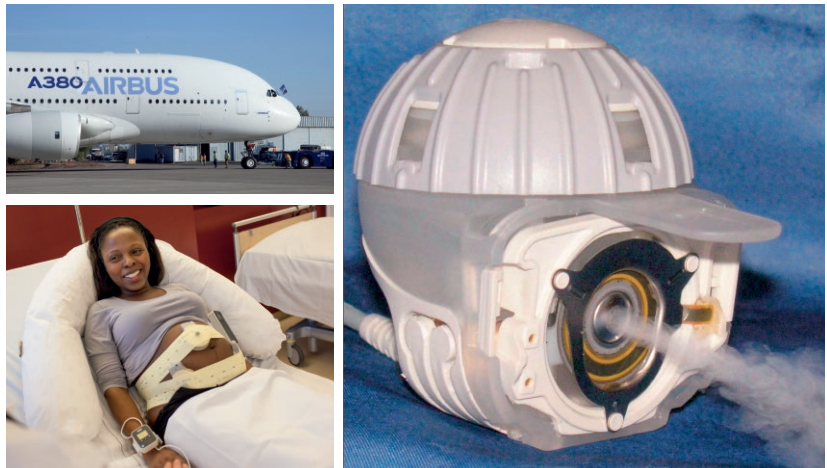
Piezoelectric sound transducers monitor the doors in the Airbus A380 (Image: Airbus, Holmco)
